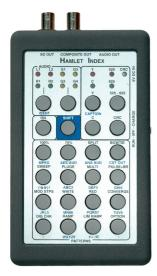
Hamlet Video International Limited, designers and manufacturers of unique digital and analog equipment produce the Protean Index for the professional broadcast industry. It is a multifunctional SD SDI, Analog, video and audio hand-held portable generator. It outputs 16 SD SDI; 16
