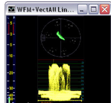
W/V – Waveform and Vector Display
